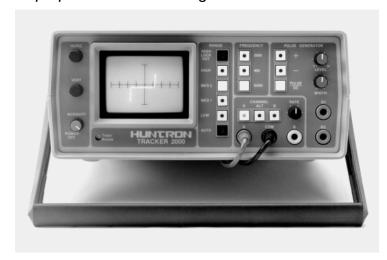
The Huntron Tracker 2000 provides advanced troubleshooting capabilities to simplify testing newer technology components such as CMOS and MOS circuits. Its built-in pulse generator lets you thoroughly troubleshoot gate-fired devices such as SCRs, TRIACs and optocouplers. By energizing the gate, you can test a component in an active mode.
